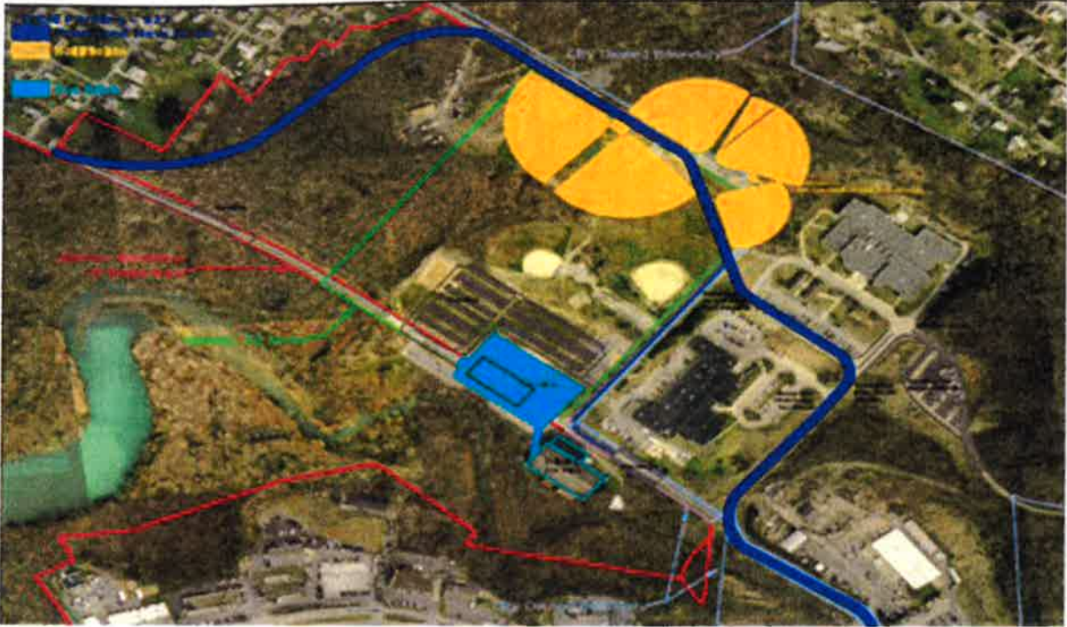
Figure 3: Proposed plan for Morgantown Recreation Center and Ice-Plex (light blue) with reconfigured ball fields (yellow) and redirected traffic (blue line) (Google Maps)
